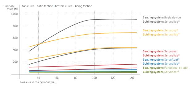
Values measured at the double-rod cylinder (seal less bore 46 mm, piston rod Ø 40 mm) in sine operation according to VDMA 24577 at 50° C/HLPD46. The friction force curves are at a lower level than is customary in the market.
